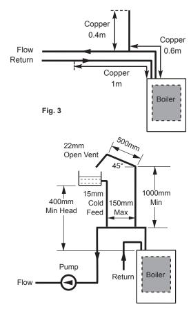
Fig. 4 Typical Low Head Installation
