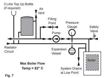
Method of determining minimum valve of expansion vessel volume for sealed systems using Baxi Boilers
