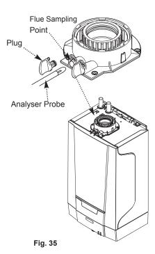
After refitting the sampling point plug ensure there is no leakage of products!
