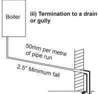
Pipe must terminate above water level to but below surrounding surface. Cut end at 45°
