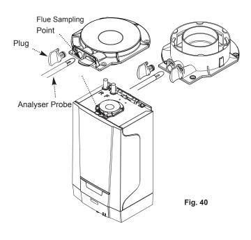
After refitting the sampling point plug ensure there is no leakage of products !
