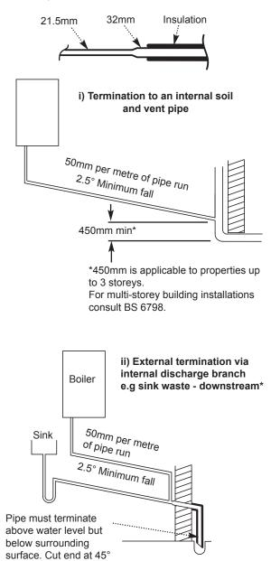
\*It is NOT RECOMMENDED to connect upstream of the sink or other waste water receptacle !
