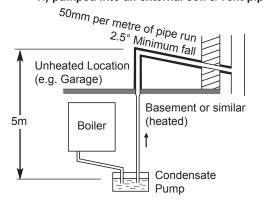
9. If the boiler is fitted in an unheated location the entire condensate discharge pipe should be treated as an external run and sized and insulated accordingly.
