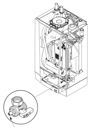
7.5.1 Check the Operational (Working) Gas Inlet Pressure
