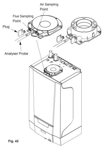
After refitting the sampling point plug ensure there is no leakage of products !
