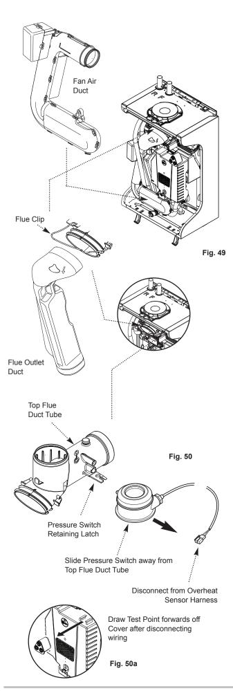
Removal of the fan air duct and flue outlet duct is necessary to enable the changing of the pressure switch, flow temperature sensor, return temperature sensor, overheat sensor and gas valve.
