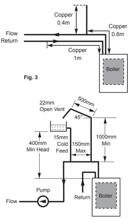
Fig. 4 Typical Low Head Installation
