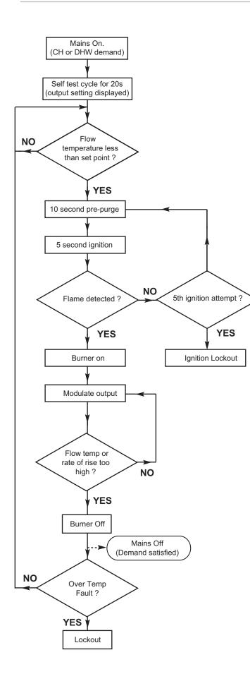
1. **Switched Live On:** When the boiler switched live turns on the boiler, a 20 second check cycle takes place. If the flow temperature is less than the boiler set-point temperature the ignition cycle will start. Pre-purge, Ignition and Burner on.
