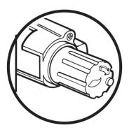
**NOTE:** The gas control knob cannot be depressed until ignition restart interlock device in gas valve has disengaged. This takes 60 seconds approximately.
