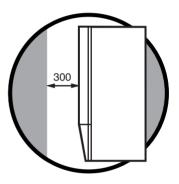
300mm is required for servicing. 5mm is required when operating.
