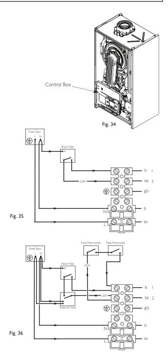
**Note:** The 230V switched signal for external controls (Frost Stat - Room Stat - Timer) must always be taken from terminal 2 at the boiler. Live, Neutral and Earth to power these controls must be taken from the Fused Spur.
