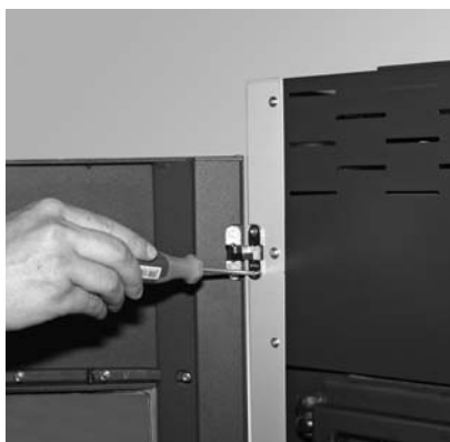
Fig. 23 Inserting the hinges in the side panel
