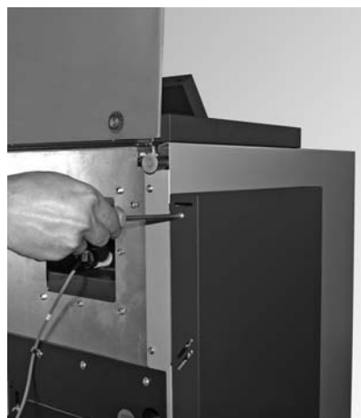
Fig. 31 Removing the securing screw
