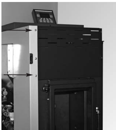
Fig. 19 Screwing the front cover plate on at the front at 2 points
